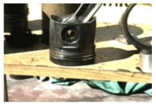
All the pistons had piston-skirts and piston rings completely clean of any build-up. The rings looked like new and did not have any wear whatsoever (very unusual phenomenon, taking into consideration that the engine was in service for 30,000 hours and had water in its oil system for more than 100 hours.)
