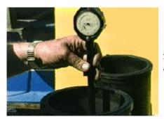
All the liners were micro-measured. There was no wear whatsoever, all the dimensions were within the manufacture's specs of a new engine.
