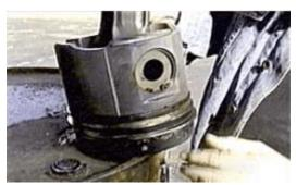
The piston-skirt and piston rings are completely clean of any deposit build-ups, and the piston ring-blades are highly polished (virtually no signs of wear). The build-up you see on the piston top, which is due to deposits from burnt fuel in combustion chamber, could be eliminated by using Bi-Tron Fuel Conditioner.
