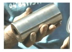
After 30,000 hours in operation and 100 hours in the presence of water, no piston pins had any traces of wear, looked shiny and new.
