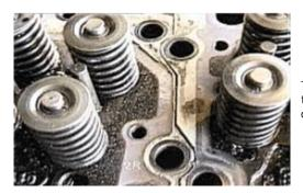
The oil baths, valve springs, valve stems and the block surface are completely clean of any deposit build-up.
